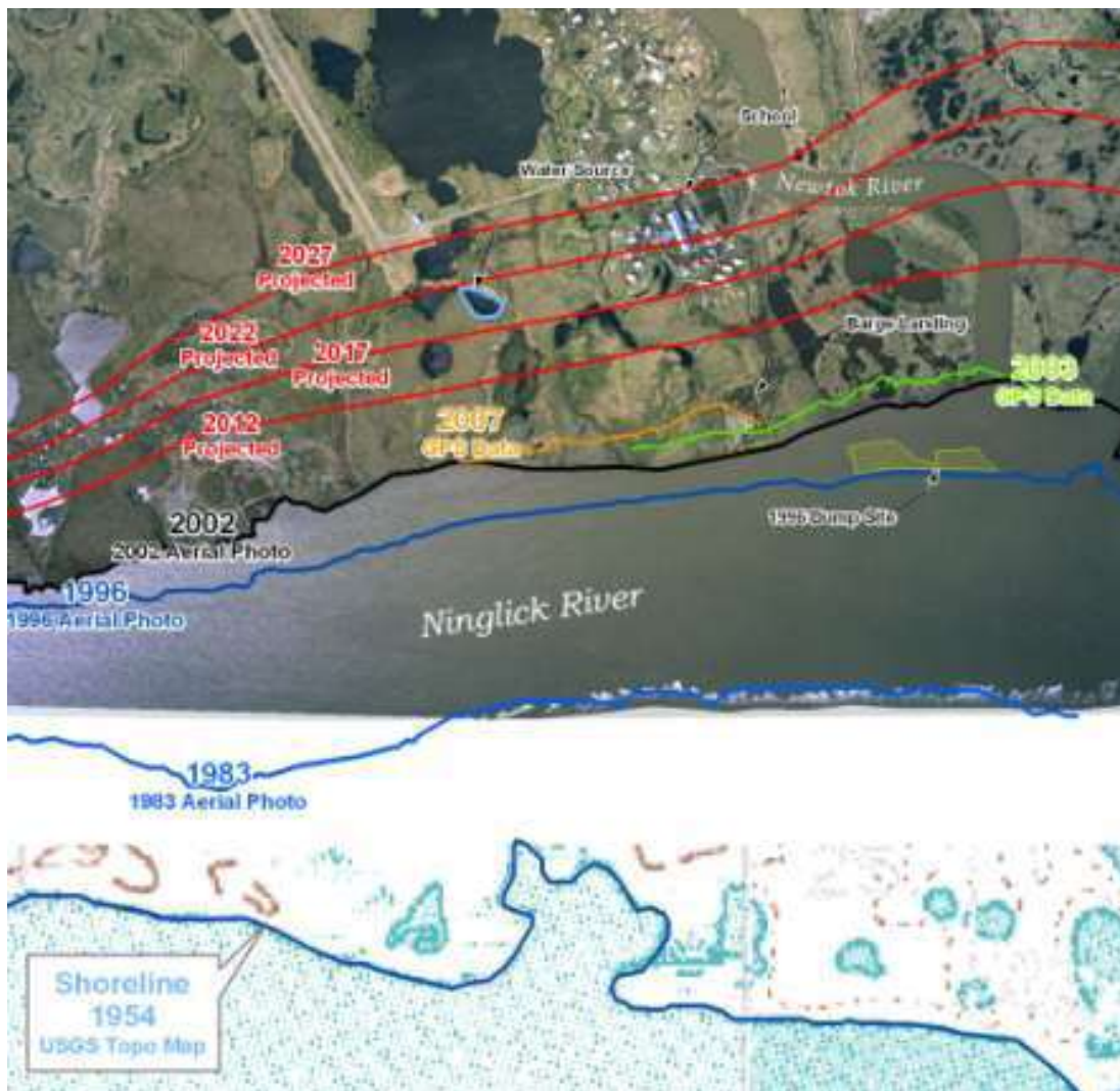
Figure 119: Past and predicted shoreline erosion for Newtok (Cook 2010)
