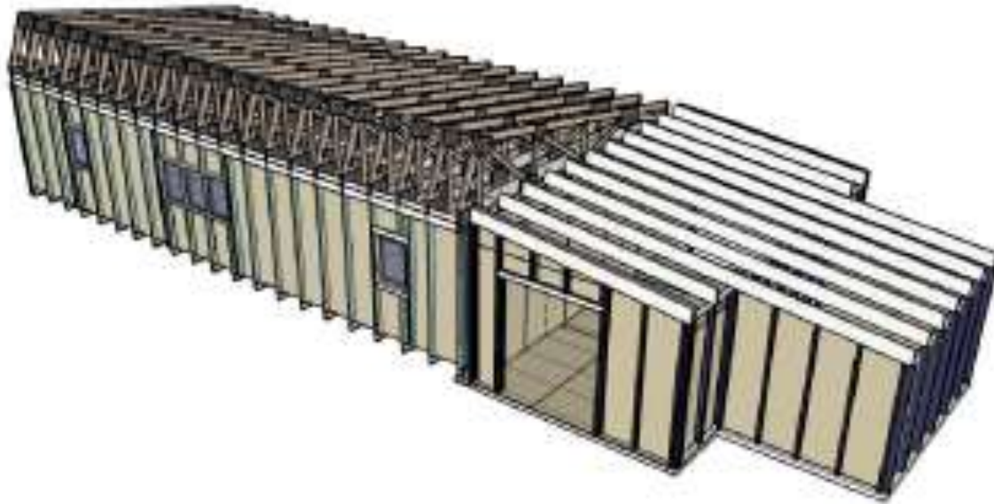
Figure 30: Steel Stud Building System (Hebert, 2010)
