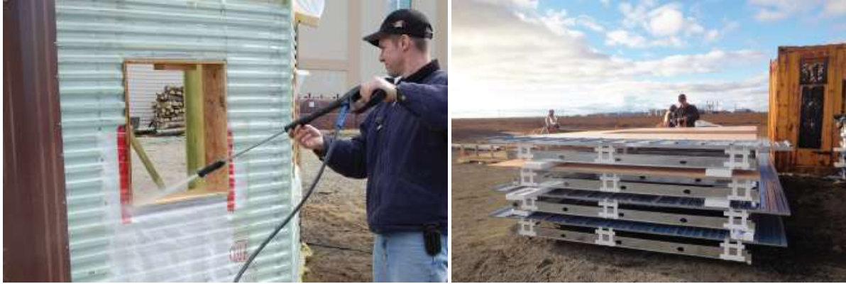
Figures 36 and 37: Wall Water Test and Assembled Wall Panels (CCHRC, 2011)
