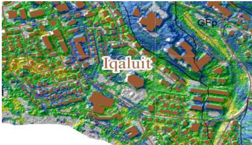
Figure 10: InSAR map created for Iqaluit by Short et al. (2012). Areas in brown show building footprints. Underneath is a layer that shows stable ground (blue), very low downward displacement (green), low downward displacement (yellow), and areas with no data (grey).
