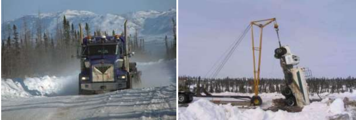
Figures 109 and 110: Winter transport (left), A truck breaks through a winter ice road (right; Semple 2009)
