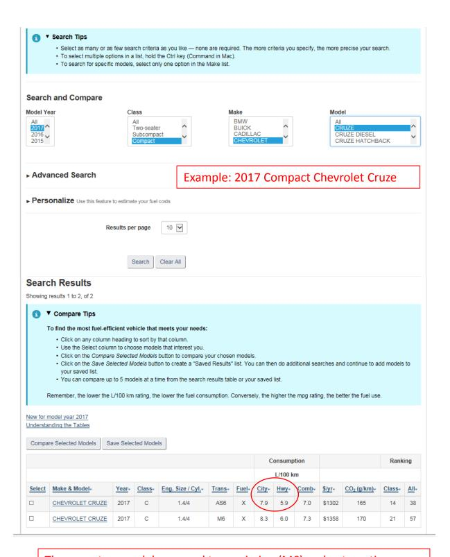
There are two models, manual transmission (M6) and automatic transmission (AS6). This example uses the automatic transmission information.
