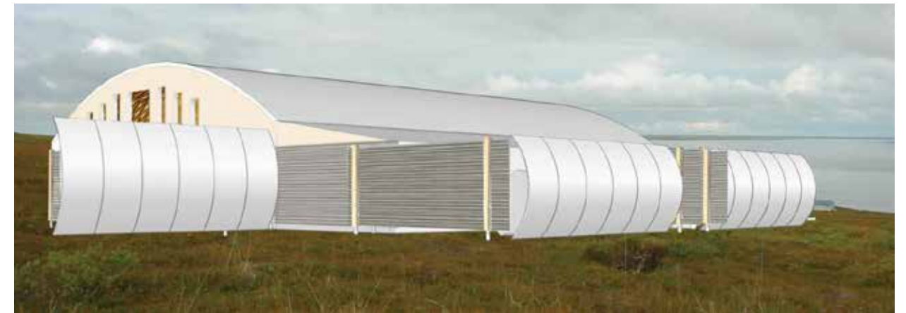
Figure 120: The aerodynamic design for the Mertarvik Evacuation Center (Cook 2010)
